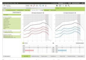
The tabs in the lower part of the screen will offer you access to the fitting tools. Each tool offers specific modifiers to fine-tune the hearing instrument
